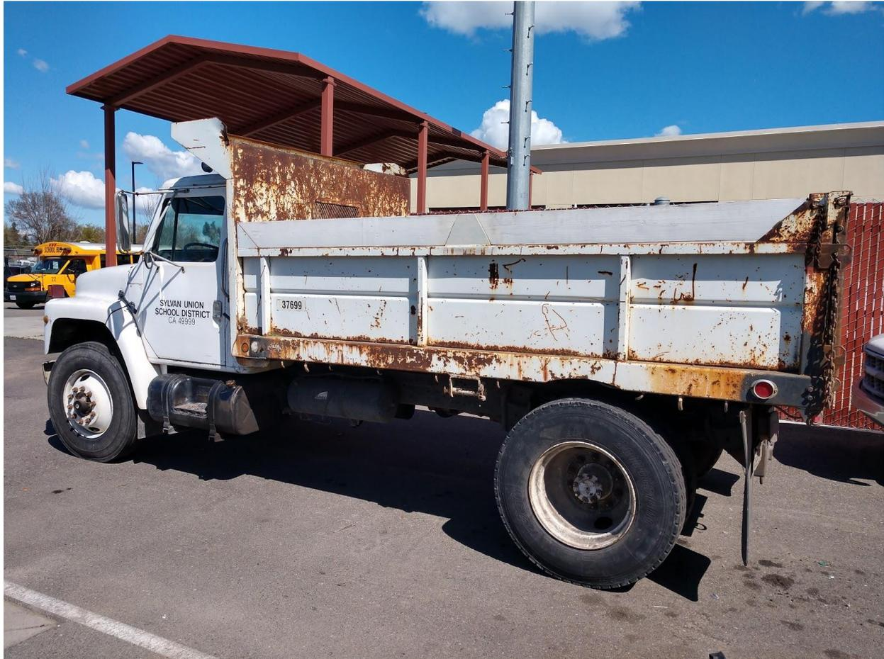
The rear bed door is unsafe to operate and has required that two people open and close when making trips to the dump or when offloading sand, wood chips or other materials at sites.
