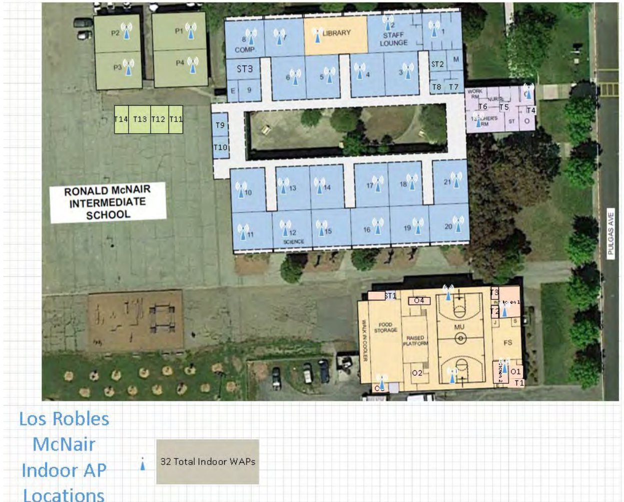
Figure 20: Indoor WAP locations at Los Robles McNair
