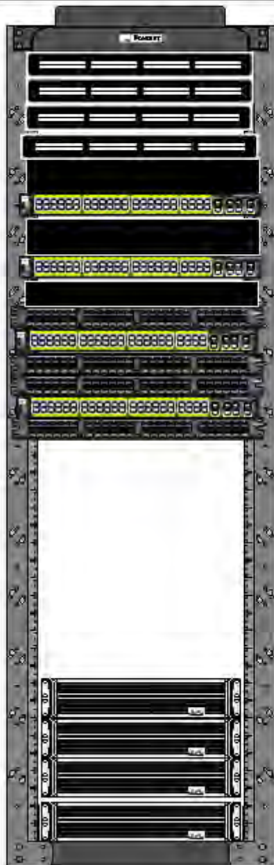
Figure 67: MDF Rack Elevation at District Offices
