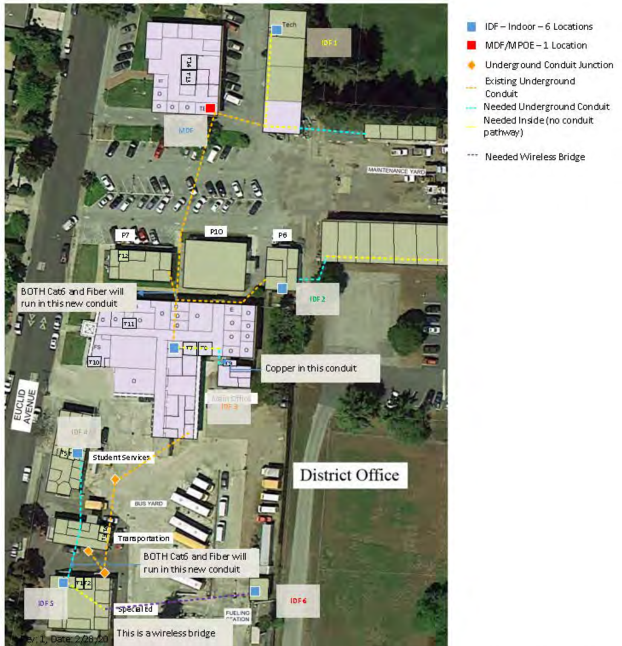
Figure 53: Cable paths and IDF Locations at District Offices
