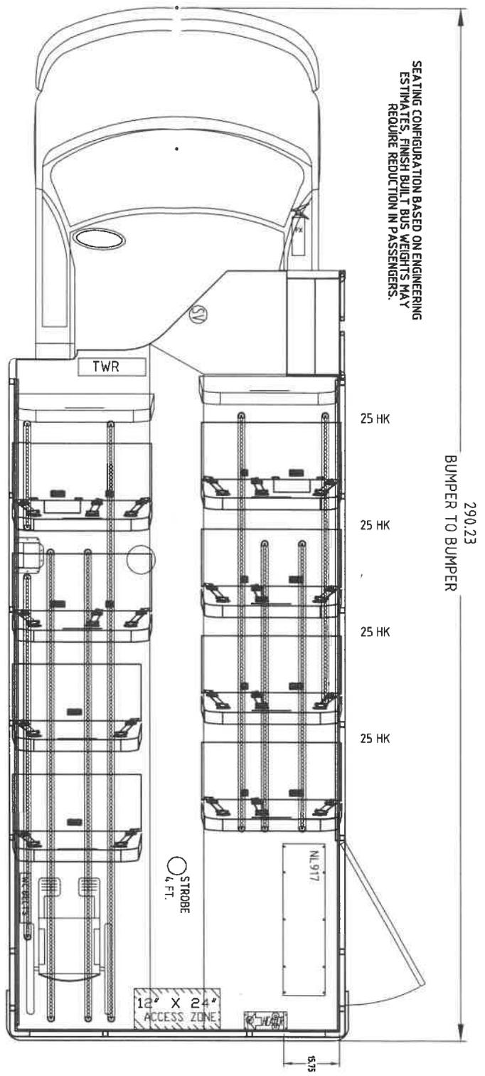
SEATING CONFIGURATION BASED ON ENGINEERING ESTIMATES. FINISH BUILT BUS WEIGHTS MAY REQUIRE REDUCTION IN PASSENGERS.
